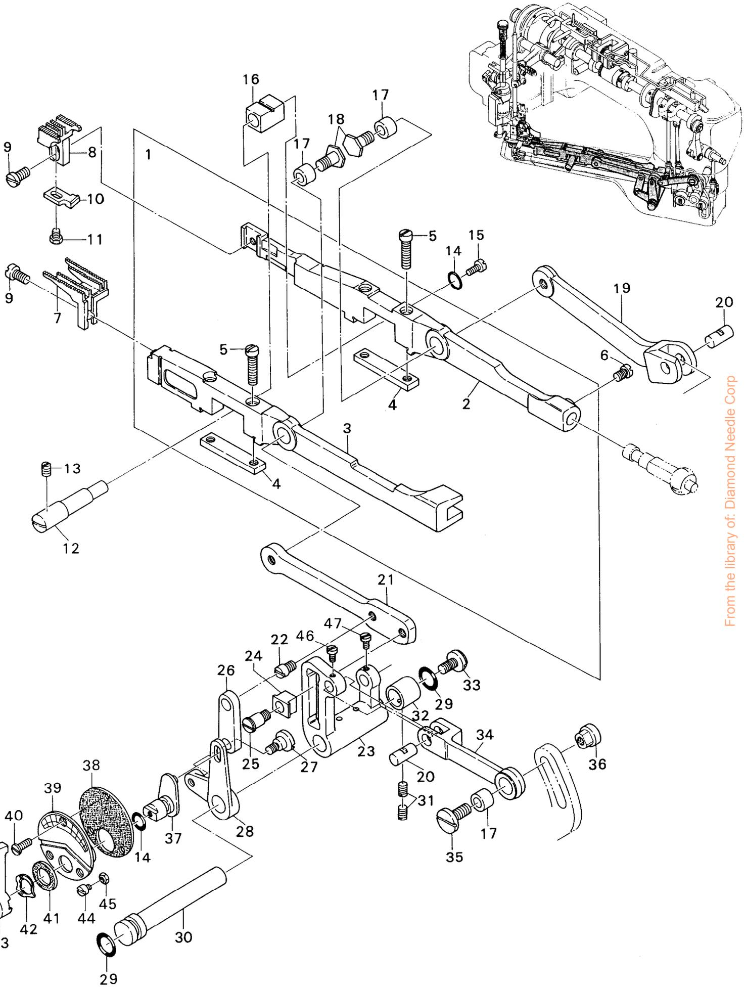
FEED DRIVING CONTROL MECHANISM
