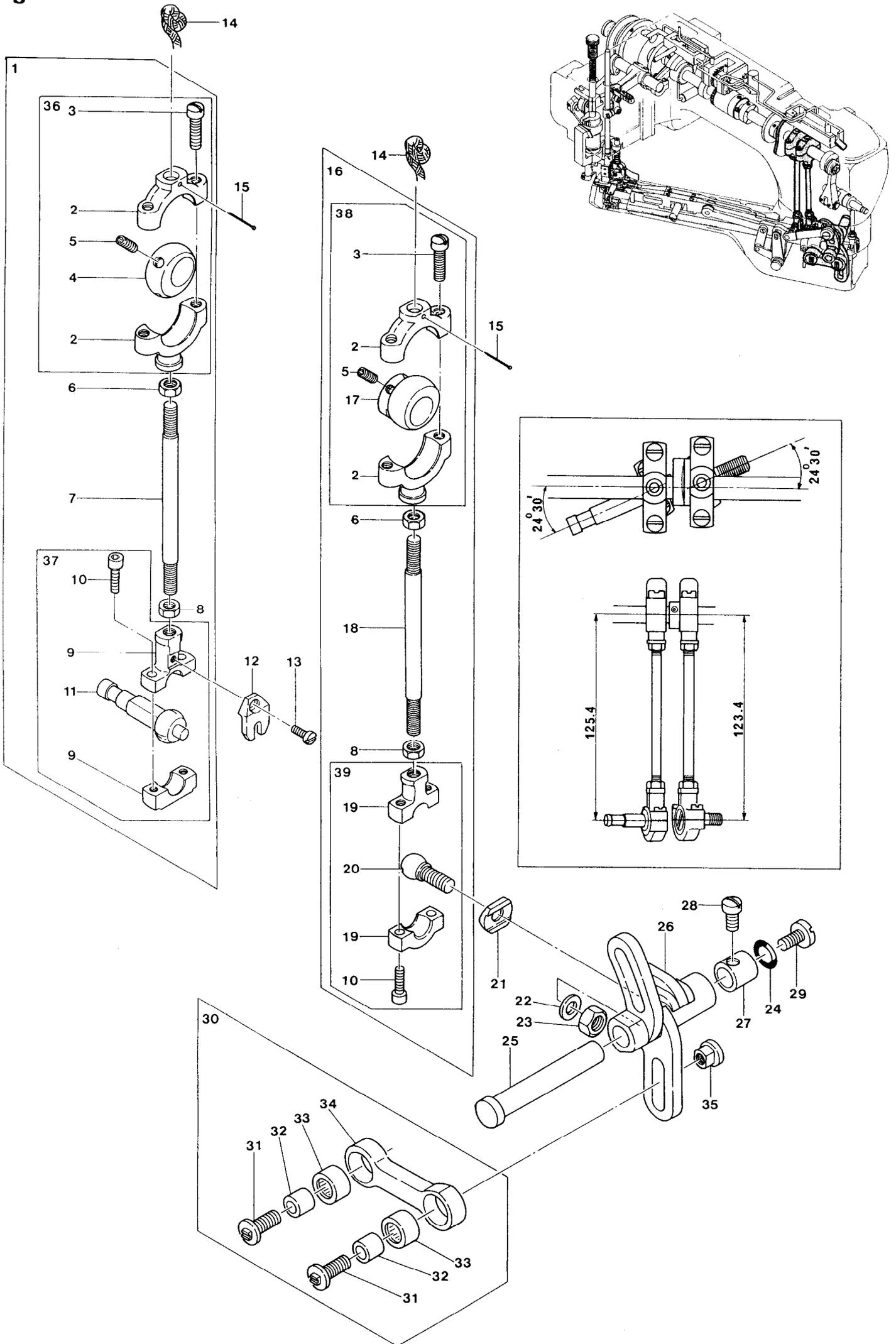
**FEED DRIVING MECHANISM**
